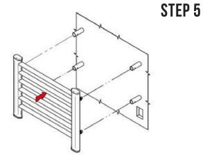
Install the towel warmer in the four connections as shown in drawing. Technical Drawings can be found on our website www.Ambaproducts.com INSTALL DIGITAL HEAT CONTROLLER OR SWITCH — SEE PAGES 6 OR 7.
