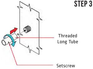
Take the threaded long tube (4) and screw it down completely to the threaded wall-support (2) ; to adjust the distance from wall unscrew tube
