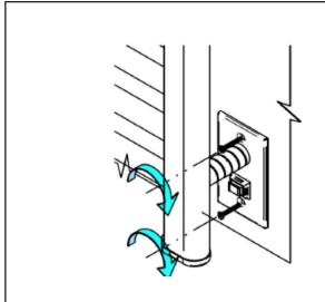
Fix the stainless steel wall-plate with the provided screws;
